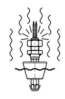
Check the water tightness between the float assembly and the cable assembly
